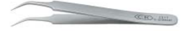
▲ 2317 SA (18/10) PRECISION TWEEZERS 105 mm 4.1/8" Fine, bent points. Finely polished. Austenitic, stainless steel, anti-magnetic and acid resistant.
