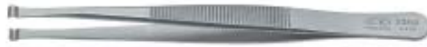
▲ 2354 SMD POSITIONING TWEEZERS TYPE 578.SA 115 mm 4.1/2" For holding, positioning and desoldering horizontal cylindrical devices up to 2 mm Ø. Tips round inside. Serrated grips.
