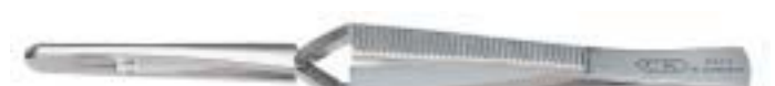
▲ 2312 C REVERSE ACTION TWEEZERS (SELF-GRIPPING) 160 mm 6.1/4" Soldering tweezers with 20 mm copper cooling jaws to absorb soldering heat. Round tips 3.5 mm. Smooth inside. Polished and fine nickel plated.
