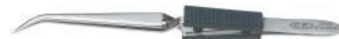
▲ 2313A C REVERSE ACTION TWEEZERS (SELF-GRIPPING) 160 mm 6.1/4" Soldering tweezers with finger pads to protect against heat. Tip width 2.5 mm, 15 mm bent. Smooth inside. Polished and fine nickel plated.
