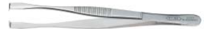
▲ 2305 C POSITIONING TWEEZERS 140 mm 5.1/2" Tip width 4.5 mm, bent 90° to inside. For extracting round and square devices. Polished and fine nickel plated. Serrated grips.
