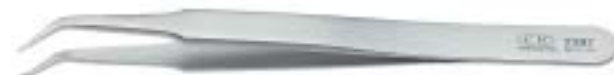
▲ 2387 SMD POSITIONING TWEEZERS TYPE SM111.SA 120 mm 4.3/4" For positioning 5 mm monolithic chip capacitors with flat base. Grooved tips, 2 mm long.
