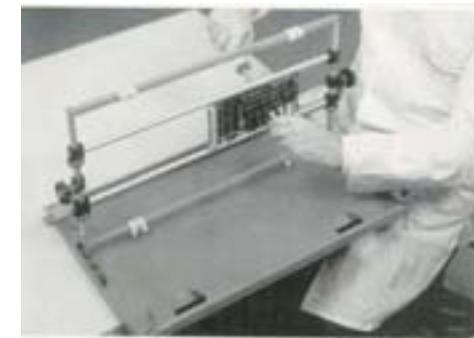
Unsoldering of components carried out with PC Assembly Jig in vertical positions.
